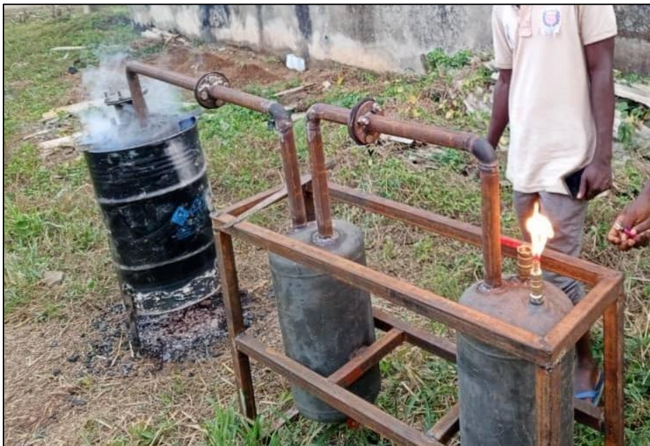
Plate 1 Pyrolysis system set-up
