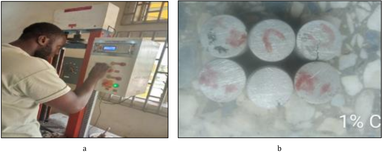
Figure 4 Compression Test using the Universal Testing Machine
