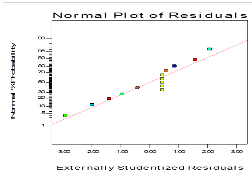
Figure 1 A graph of normal % probability against externally studentized residuals for removal of TDS in Soluos dumpsite leachate
