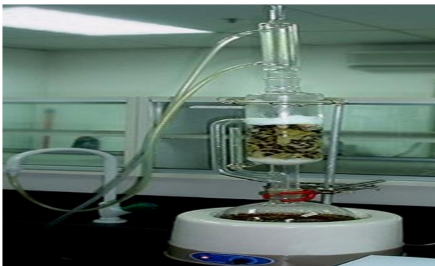
Figure 1 Extraction Process (Soxhlet apparatus)
